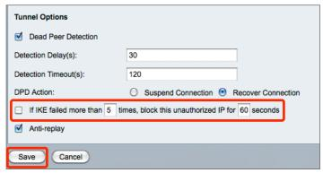
➤ To prevent you from being locked out while setting up and testing the connection, it is very important to **disable** the checkbox, **If IKE failed more** than ... times, block this unauthorized IP for ... seconds"
