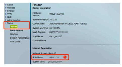
Internet Connection: Write down the IP address of your VPN gateway (here: 203.0.113.1) as ① on your → Configuration Checklist If you have a dynamic DNS (DynDNS) service set up for your router, you can write it down instead.
