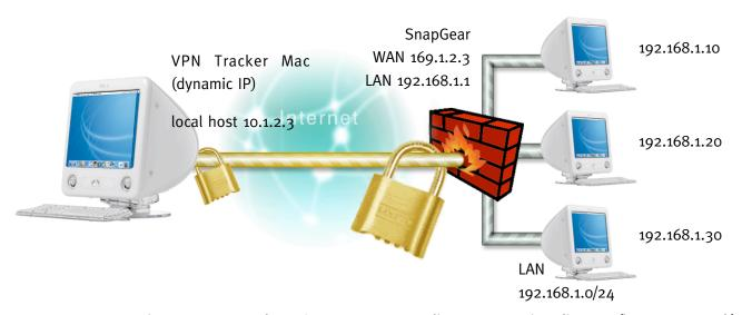
Figure 1: VPN Tracker - SnapGear VPN Appliance connection diagram (host to network)
