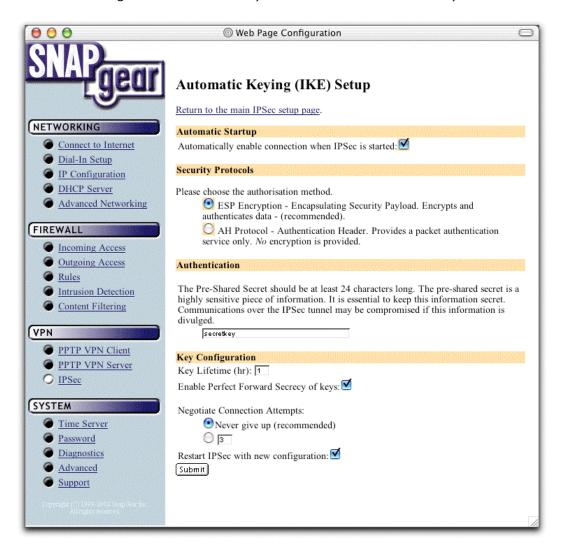
Figure 4: Automatic Keying Setup dialog
