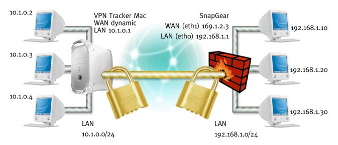
Figure 8: VPN Tracker – SnapGear connection diagram (network to network)
